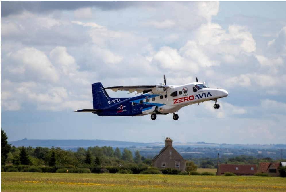
Figure 5 Retrofitted Do228 equipped with ZA 600 hydrogen-electric engine during flight test campaign (source:ZeroAvia)
